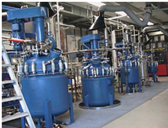
Fig. 6 Hyperthermophiles fermentation plant, University of Regensburg. Partial view, showing two 300 l and one 130 l fermentors
